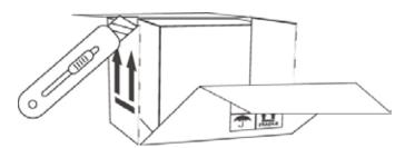
Cut down each side of the box to reveal the systems so that you don't have to lift them out of the box. Install the water heater on the right-hand side of the cupboard after you've installed the SmartTap $^{\text{TM}}$ .
