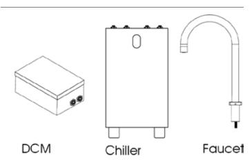
The DCM can be freestanding or we advise it to be installed on the right side wall of the sink cabinet with the chiller as close to the DCM as possible.
