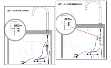
4. Decide where the tap is going to sit. Note that the control panel on the drip tray is on the right-hand side of the tap. Ensure that the location you choose is suitable and that you can reach the controls without needing to stretch while ensuring that the user will not have to reach through the stream of water to operate the tap.
