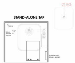
5. The tap can be fitted either to the side of the sink or at the back of the sink. Before you start cutting, ensure that you have set up a jig or a template device to prevent the drill bit from moving when you cut.
