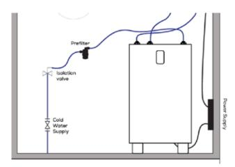
2. Connect the blue  $\frac{1}{4}$ " tube found in the installation kit to this  $\frac{1}{4}$ " connection on the mains supply (push in firmly and fit  $\frac{1}{4}$ " red locking clip), then cut it at a length that extends to the front of the cupboard where the chiller inlet will sit. Install isolator making sure it is closed.
