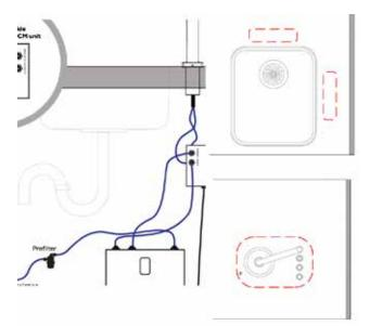
THE COMMS CABLE CONNECTS INTO THE SIDE OF THE DCM. THE DCM MUST BE LOCATED CLOSE TO THIS CABLE WITHOUT CAUSING IT TO STRETCH.
