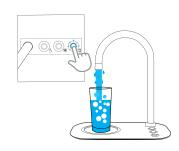
Between adjustments, eral glasses of sparkling water to see the effects of the adjustment. If the sparkling function is spluttering, there is too much gas in the water. Reduce the setting by one full turn and try again.
