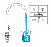
Between adjustments, you must run off several glasses of sparkling water to see the effects of the adjustment. If the sparkling function is spluttering, there is too much gas in the water. Reduce the setting by one full turn and try again.
