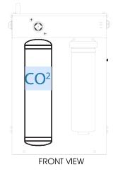
To decrease the level of carbonation, turn the regulator by a half turn in a counter-clockwise direction.
